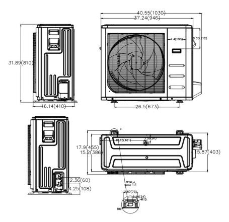
Drawing dimensions are nominal. **4**. It is not recommended to exceed 125% connected capacity. Maximum output of the system is dictated by the outdoor unit; connected capacities beyond maximum output of outdoor unit will not result in increased system output. Refer to full product literature for allowable combinations of units. **5**. Connection of these accessories may require secondary items not listed; refer to full product literature. | Specifications subject to change without notice.
