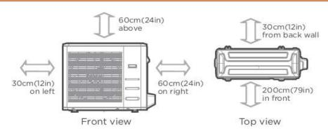
Note: Outdoor units must be elevated 12-24in. (30.5-61cm) above the surface below in heating applications to allow for snow clearance and defrost runoff. Follow local best-practices and guidelines.
