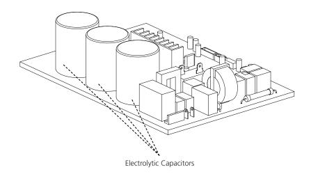
For other models, connect discharge resistance (approx.100 $\Omega$  40W) or a soldering iron plug between the positive and negative terminals of the electrolytic capacitor. The terminals are located on the bottom surface of the outdoor PCB.
